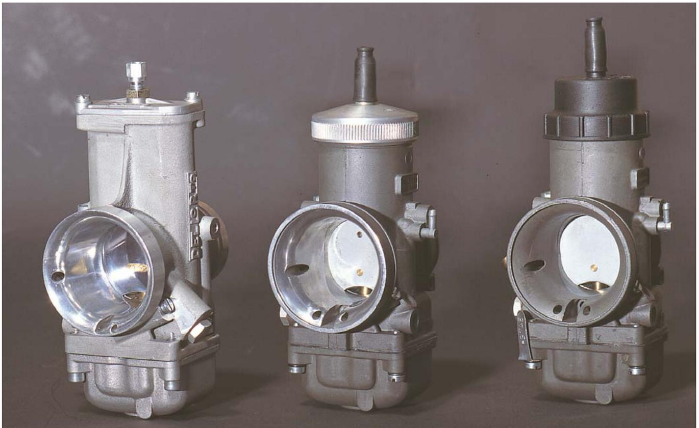
The venturi of the modern motorcycle carburetor is carefully developed to reduce disturbances in the flow around the throttle valve and its seat.
